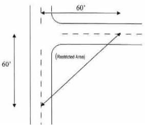
Corner lot development and planting is restricted in the triangular area formed by the sight-line between points in the two street centerlines, 60 feet from the center of the intersection
